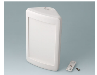
B4610207 SMART-CONTROL M, Vers. II ASA+PC-FR (UL 94 V-0) off-white RAL 9002 173x101x59mm IP 55 opt., IP 40
