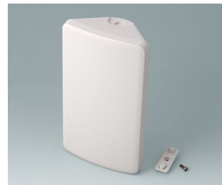
B4610107 SMART-CONTROL M, Vers. I ASA+PC-FR (UL 94 V-0) off-white RAL 9002 173x101x59mm IP 55 opt., IP 40
