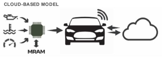
1 Sensor Fusion combines multiple sensor inputs into packets
